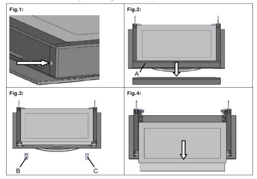
Method 2 remove and assemble procedure:
